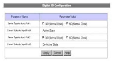
door switch might be normally closed but open in response to an opened door, or it might be normally open but close in response to an opened door. This menu allows the administrator to specify which state matches the actuated or triggered position of the sensor. See details in Appendix 7 for specific wiring requirements for your sensor and detailed information about using these settings.
